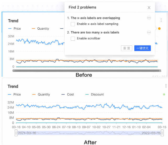
Fig. 5. An instance of using Linter to find and fix problems in a line chart.
